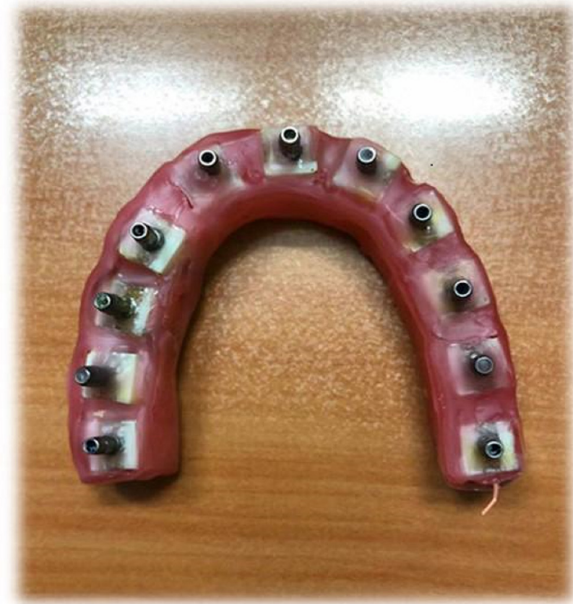
Figure 3: The boxes were fabricated in the shape and form of a mandible using five layers of red dental wax.
